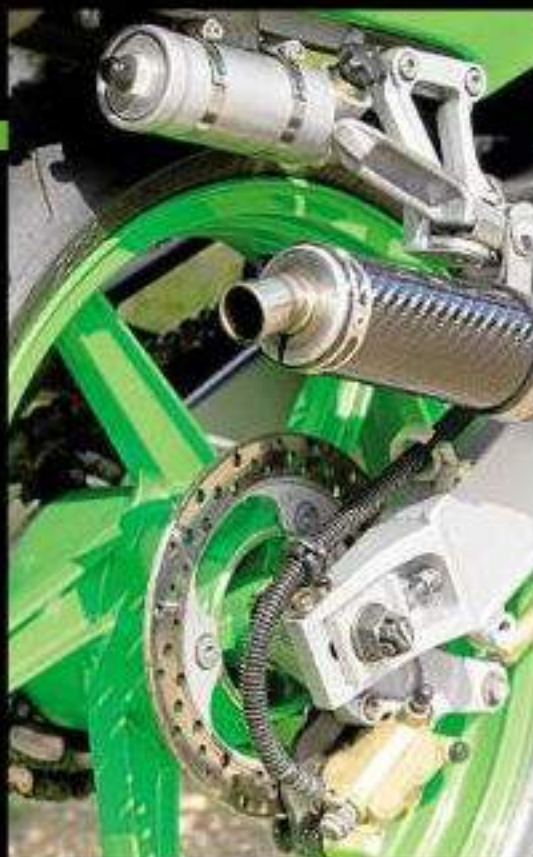
140-section rear limits tyre options
