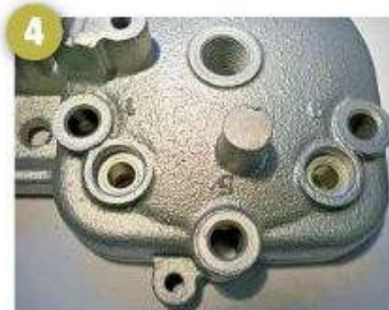
Bushes prevent the KIPS valves rattling
