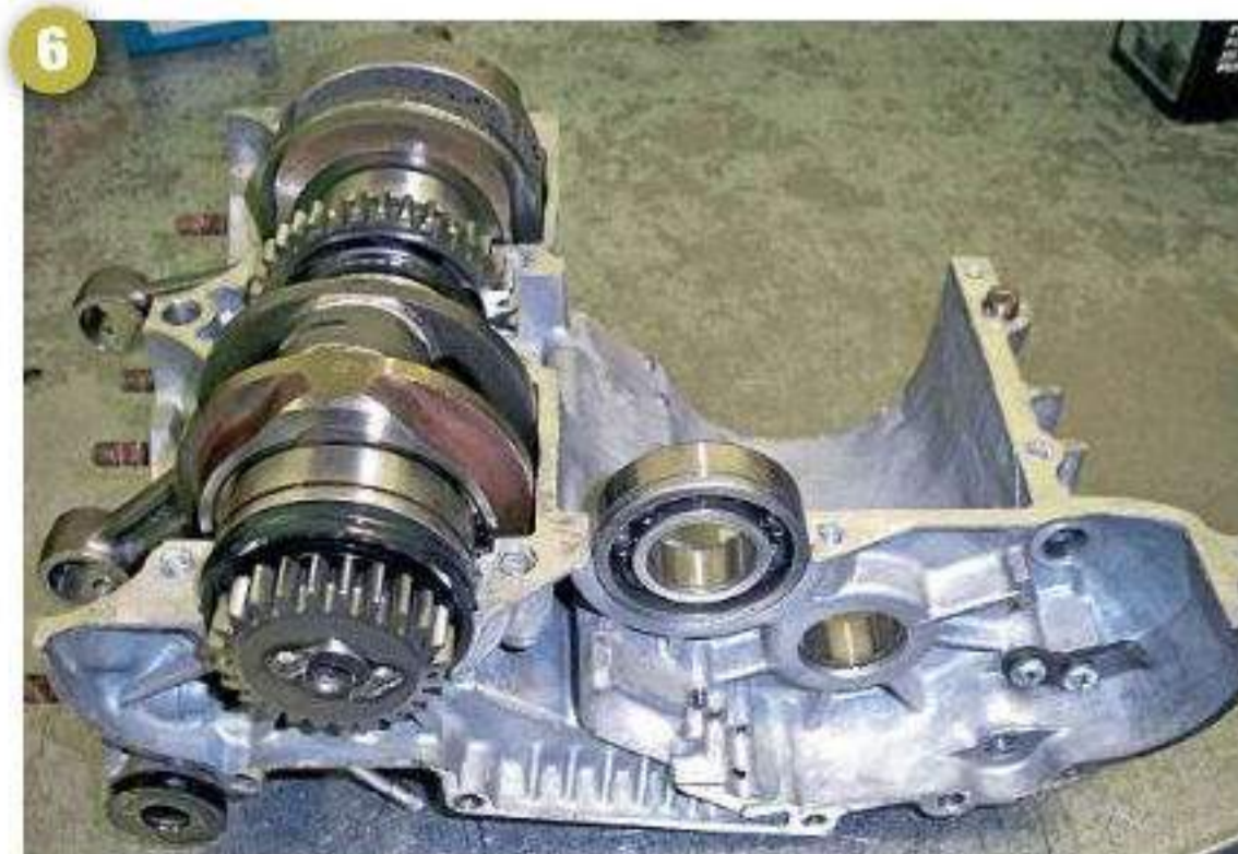
Gearbox bearing must be fitted when assembling the crank cases
