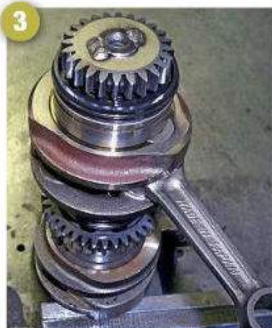
Primary gear is tack-welded on
