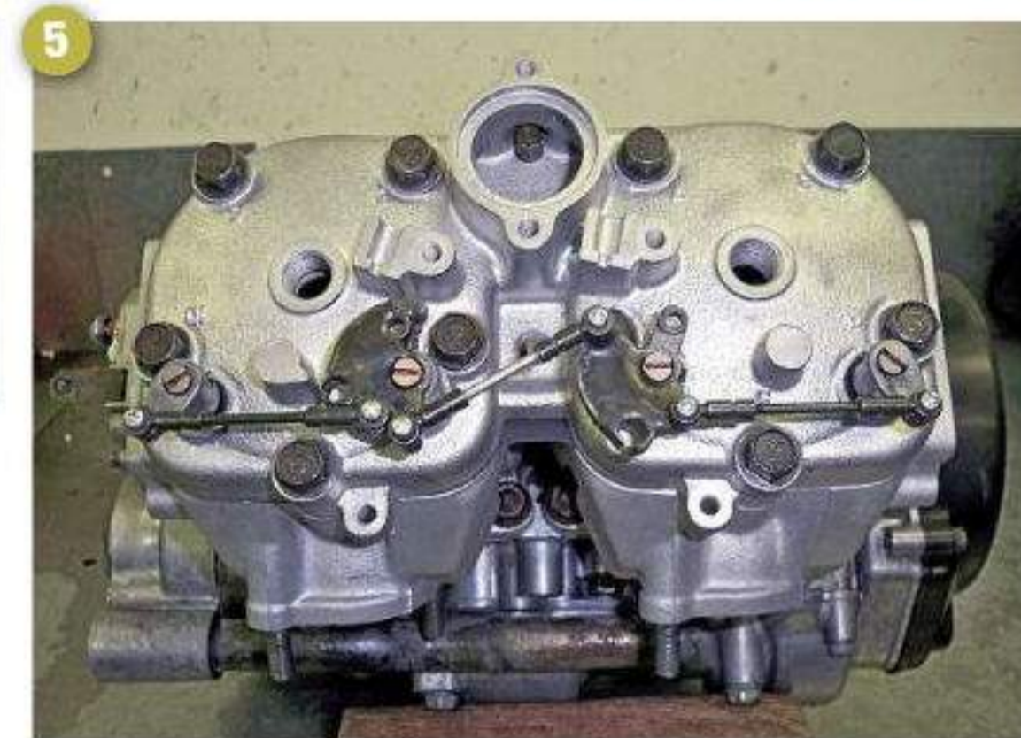
This is how the KIPS linkage should look upon reassembly
