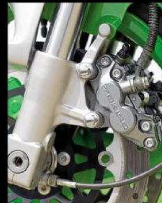
Forks are adjustable for rebound and preload
