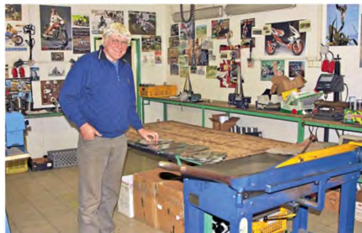
Jim Lomas in the cutting room. This is where the individual cone patterns are scribed and cut
