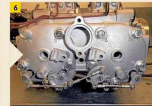
1/ Here are the exhaust boost ports shut 2/ This shows the KIPS port open. 3/ And now the exhaust boost ports open. 4/ This is the KIPS port shut. 5/ Here we see the KIPS linkage closed... 6/ ...and the KIPS linkage open.
