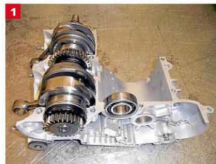
1/ Here we have the gearbox bearing and crank in the top crankcase. 2/ You can see the crank gear balance marks. 3/ Here are the balance shaft marks. Simple when it's all on display.
