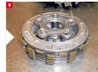
7/ Now we're sliding in the cassette gearbox. 8/ Idler gear, oil feed, shaft clip and shim, doing their thing. 9/ This is the clutch plate pack loosely assembled and ready to go.
