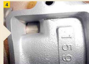
1/ Here are the exhaust boost ports shut 2/ This shows the KIPS port open. 3/ And now the exhaust boost ports open. 4/ This is the KIPS port shut. 5/ Here we see the KIPS linkage closed... 6/ ...and the KIPS linkage open.
