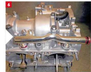
4/ Not my best shot, a poor photo of the marks lining up. Sorry, but I do my best for you! 5/ Here you see the balance shaft and oil feed. 6/ And here we have the steel water pipe and rubber oil pipe.
