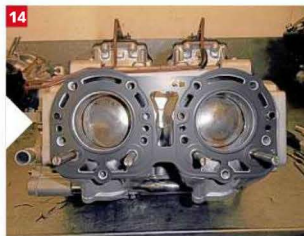
13/ Now to squeeze the rings into the grooves and slide the barrel on. 14/ We're now all ready for the head. 15/ We're checking squish with solder because the barrels had been shortened.
