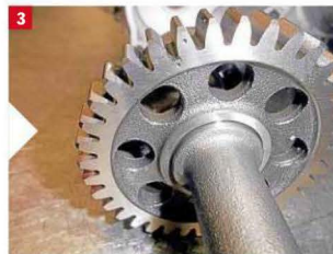
1/ Here we have the gearbox bearing and crank in the top crankcase. 2/ You can see the crank gear balance marks. 3/ Here are the balance shaft marks. Simple when it's all on display.
