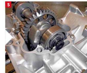
4/ Not my best shot, a poor photo of the marks lining up. Sorry, but I do my best for you! 5/ Here you see the balance shaft and oil feed. 6/ And here we have the steel water pipe and rubber oil pipe.
