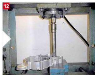
10/ This is the completed right-hand side of the KR-1S motor all assembled. 11/ All the water pump parts laid out for your delection. 12/ Now here you see us pressing in the water pump seal.
