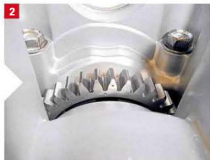
1/ Here we have the gearbox bearing and crank in the top crankcase. 2/ You can see the crank gear balance marks. 3/ Here are the balance shaft marks. Simple when it's all on display.
